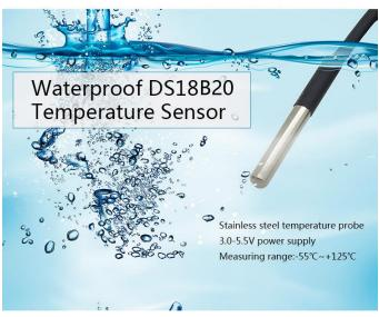
We are selling two kinds of sensors: AM2301 and DS18B20(measures temperature only). We've customized an interface for Sonoff TH10/TH16 to easily connect with the sensor-just plug and play. Note that the sensor should be plugged before power up. It is not advised to plug or unplug the sensor in power on state. Furthermore, AM2301 is non-waterproof, while DS18B20 is waterproof.
